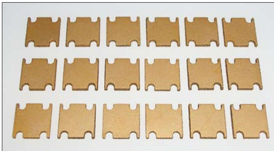
Nano Materials International's aluminum-diamond matrix composites have thermal conductivity greater than 500 W/m-K, compared with about 200 W/m-K for copper-tungsten or copper-moly-copper.
