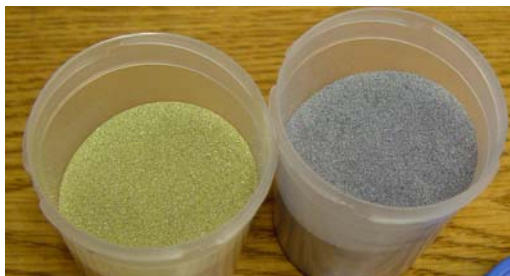
Figure 3. Non-converted (left) and SiC converted (right) diamond powder (coarse particle size shown).
