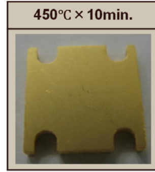
Figure 6. Ni/Au plated aluminum diamond sample after bake test (no visual blisters observed)
