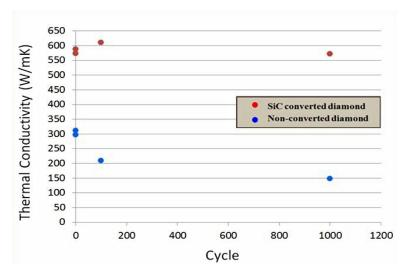
2. Test results of SiC surface-converted and non-surfaceconverted diamond powder after 10 cycles at 500° C for 1 hr., Note degradation of non-converted powder.
