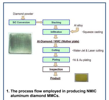
The literature contains the results of these efforts using diamond and a variety of metals, but development at NMIC showed that aluminum appeared to be an excellent choice. MMCs in general combine a primary metal such as aluminum or copper in combination with diamond (silicon carbide has also been used).
